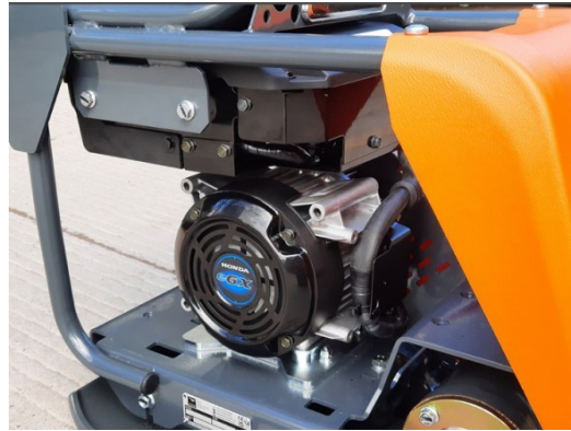
Emission free, low noise, battery powered Honda eGX motor.
