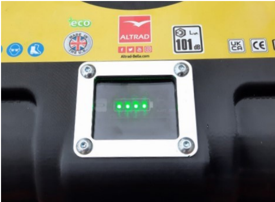
Battery power level indicator.
